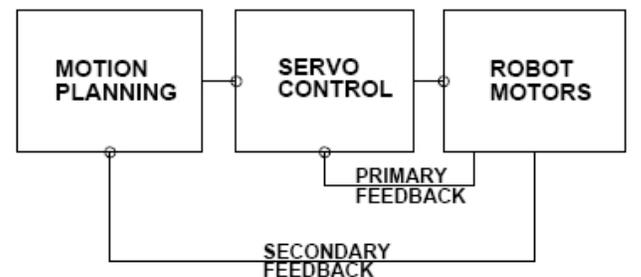
**Figure 6.** Secondary feedback sent to motion planner
