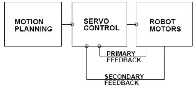
**Figure 5.** Direct use of secondary feedback
