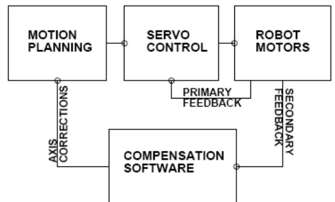
**Figure 7.** Secondary feedback collected and conditioned via software program, then sent to motion planner
