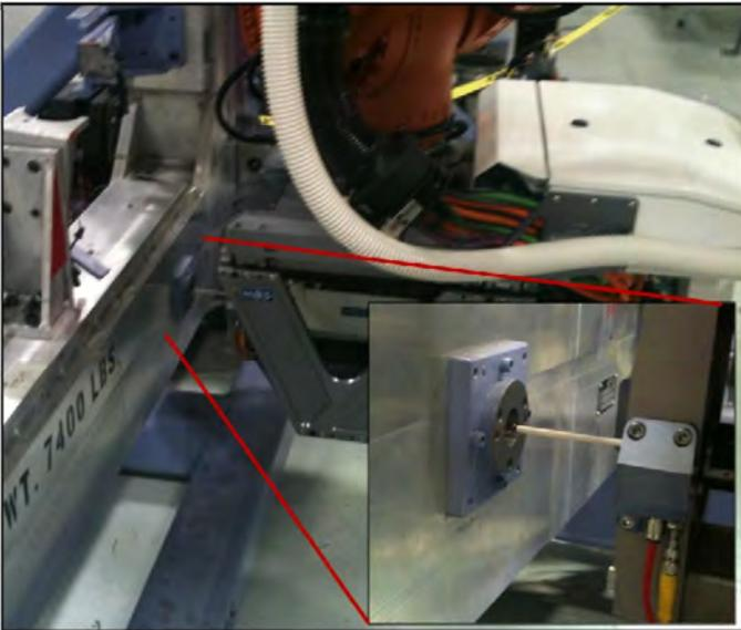
**Figure 6. Wireless touch probing of fixture targets**
