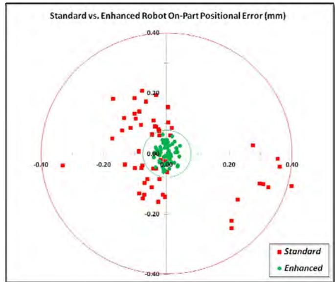
**Figure 3. Accuracy comparison: Standard vs. Enhanced**
