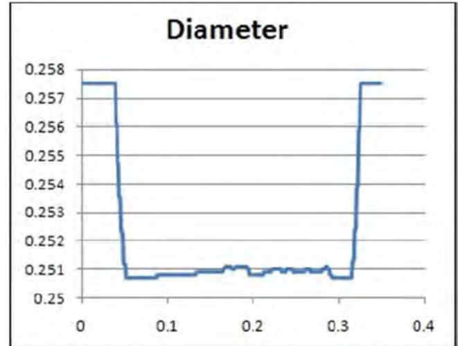
**Figure 8. Hole profile data collected by probe**
