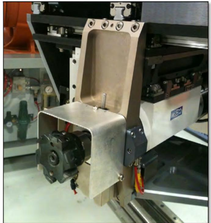
**Figure 9. 76mm end mill and shroud for face milling operations**
