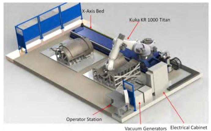
**Figure 4. Overall Cell Layout**
