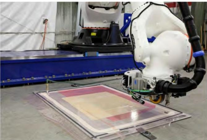
**Figure 3. Robot and EE working on a test panel**
