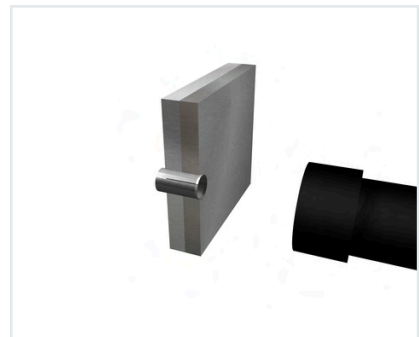
09 Retract mandrel fully into the nose cap
